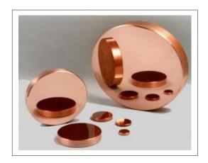
High energy lasers require the best mirrors available. Uncoated copper mirrors by SPAWR offer the highest quality and surface damage threshold available for medium and long wave IR lasers. High reflectance coatings on these mirrors are typically not required, however, they are available as a vacuum deposited protected silver coating or an electro chemically deposited hard gold coating.
